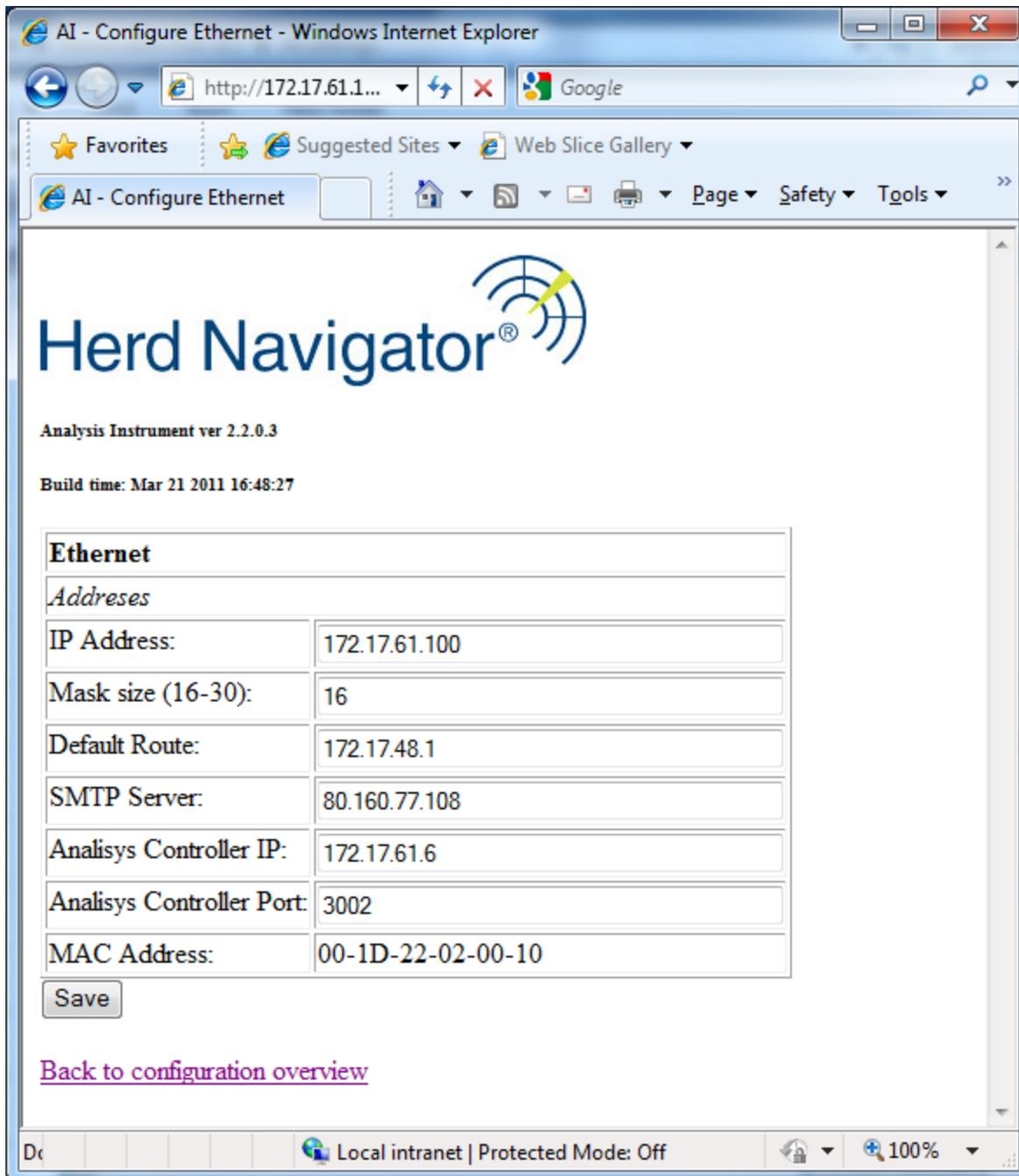
Enter the IP for the AC in the Analysis Controller IP field, and if there is more than one AI, change Analysis Controller Port, normal installations use 3002. Remember to save the new settings.
