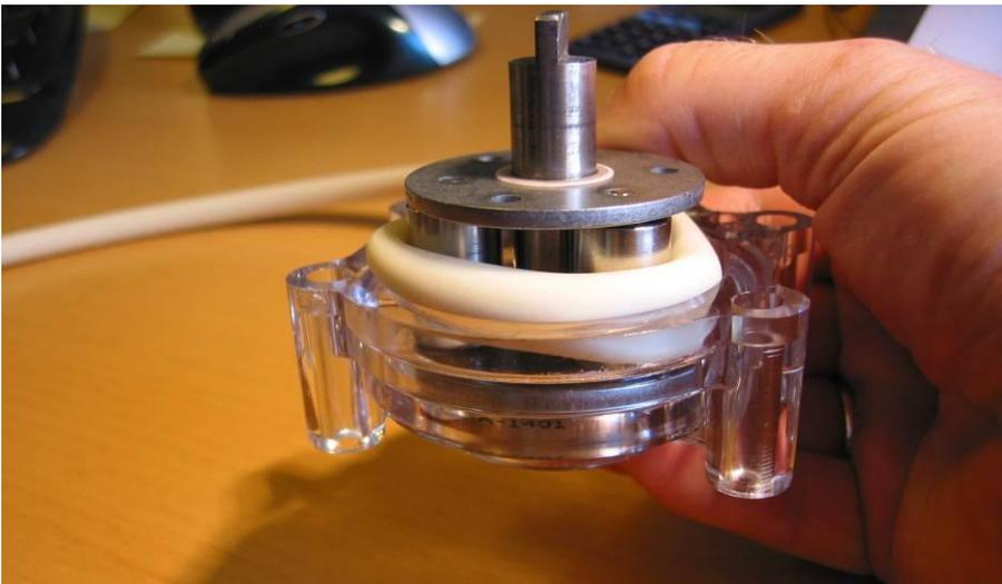
Check the length of the tube on the pressure side, it should be 100 mm. Mount the pump housing on the motor shaft and fit the 4 screws holding the housing to the motor. The other end of the tube should be fitted as shown on the later pictures.
