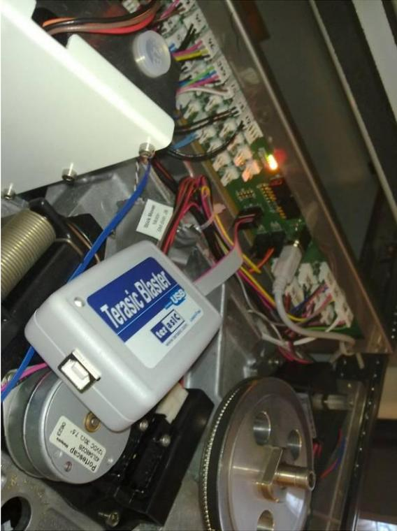
**Figur 3 : Connect USB Blaster (Red line in top)**
