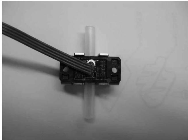
Remove the protective tape from the foam pad and glue it onto the detector. Make sure that the holes in pad and bracket are centered.
