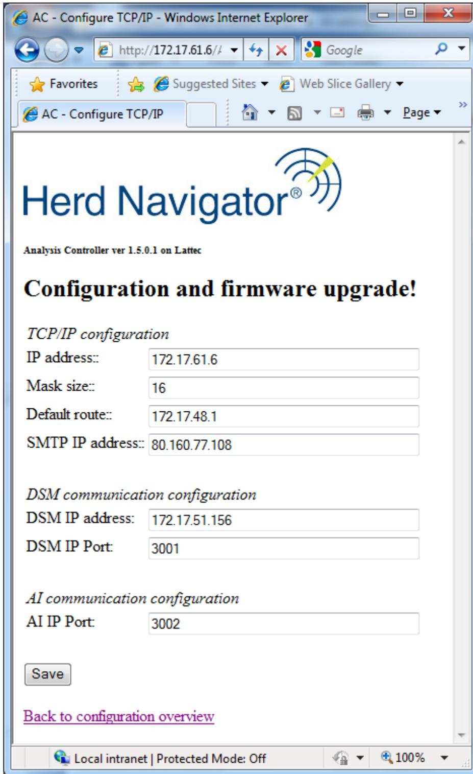
Make sure the AI IP Port is the same as in AI settings, standard = 3002 , Remember to save if changes are made.
